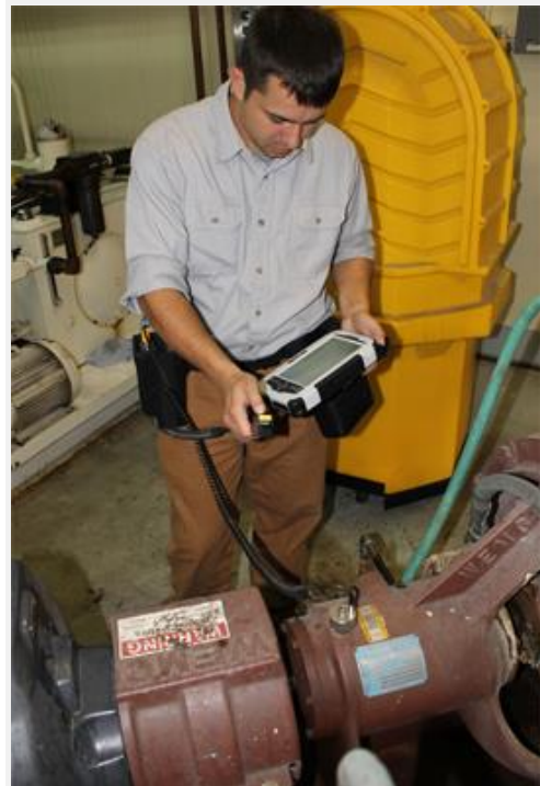
Figure 3. Vibration monitoring can be used to analyze the mechanical condition of rotating machinery and as a detection method for all classes of mechanical faults.
