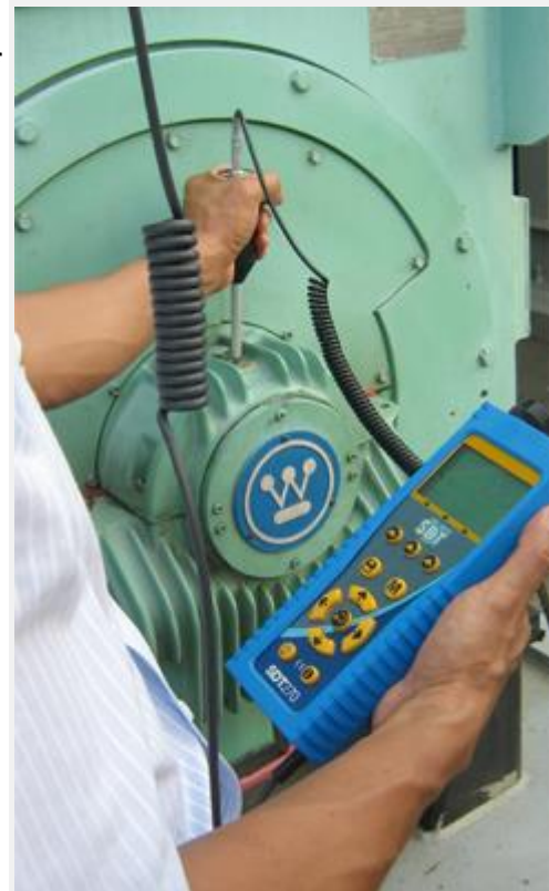
Figure 2. Capturing dynamic ultrasound data on the non-drive end bearing of electric motor gives an indication of over- or under-lubrication and possible early stage fault condition.
