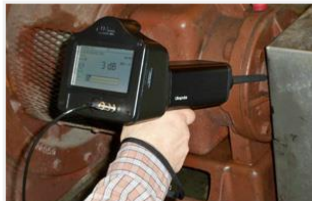
Figure 1. Utilize ultrasound as the primary tool for monitoring bearing condition.
